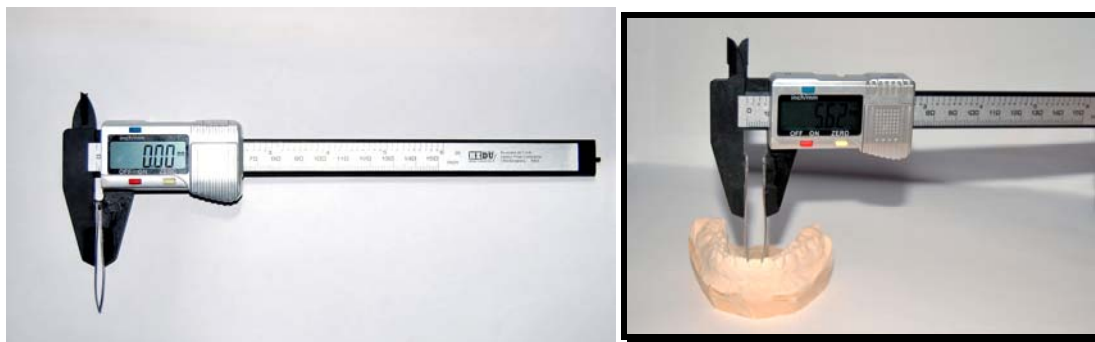
Figure 1. Digital caliper modified with two wipla rods 0.8mm diameter and 5cm length. Lower central incisor measurement with modified digital caliper Hedü
